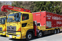
Large-capacity pumping trucks
