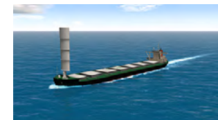
Simulation of a coal vessel equipped with Wind Challenger equipment
