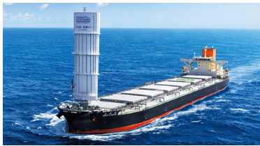
Reducing the environmental impact of fuel transport through introduction of Shofumaru, the world's first coal transport ship equipped with Wind Challenger technology Fuel conservation Results Up to 17% (per day) Average 5-8% (per trip)
