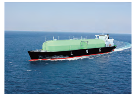
This new LNG carrier slated for the U.S. Cameron project is a 165,000m 3 type LNG carrier. (Photo courtesy Mitsubishi Heavy Industries Shipbuilding Co., Ltd.)
