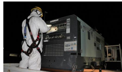
Nighttime training for securing fuel for emergency diesel power generators during severe winters (Higashidori)
